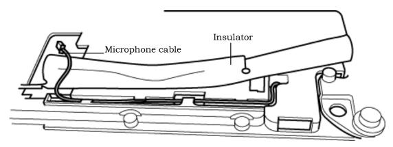
Figure 4-20 Removing the microphone cable
